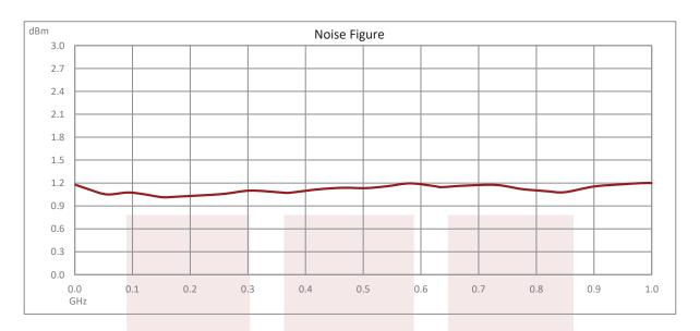
1 dB NF Input Protected Low Noise Amplifier, Operating from 0.001 MHz to 1 GHz with 40 dB Gain, 15 dBm P1dB and SMA from Fairview Microwave is in-stock and available to ship same-day. All of our RF/microwave products are available off-the-shelf from our ISO 9001:2008 certified facilities in Lewisville, Texas. Fairview Microwave is RF on-demand.
