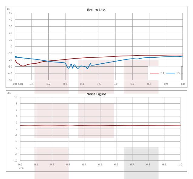
1 dB NF Input Protected Low Noise Amplifier, Operating from 0.001 MHz to 1 GHz with 60 dB Gain, 16 dBm P1dB and SMA from Fairview Microwave is in-stock and available to ship same-day. All of our RF/microwave products are available off-the-shelf from our ISO 9001:2008 certified facilities in Lewisville, Texas. Fairview Microwave is RF on-demand.
