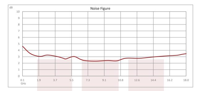
3 dB NF Input Protected Low Noise Amplifier, Operating from 100 MHz to 18 GHz with 38 dB Gain, 19.5 dBm Psat and SMA from Fairview Microwave is in-stock and available to ship same-day. All of our RF/microwave products are available off-the-shelf from our ISO 9001:2008 certified facilities in Lewisville, Texas. Fairview Microwave is RF on-demand.
