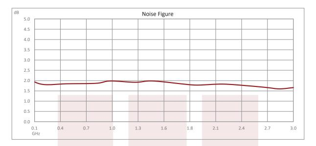
1.7 dB NF Input Protected Low Noise Amplifier, Operating from 30 MHz to 3 GHz with 30 dB Gain, 15 dBm P1dB and SMA from Fairview Microwave is in-stock and available to ship same-day. All of our RF/microwave products are available off-the-shelf from our ISO 9001:2008 certified facilities in Lewisville, Texas. Fairview Microwave is RF on-demand.
