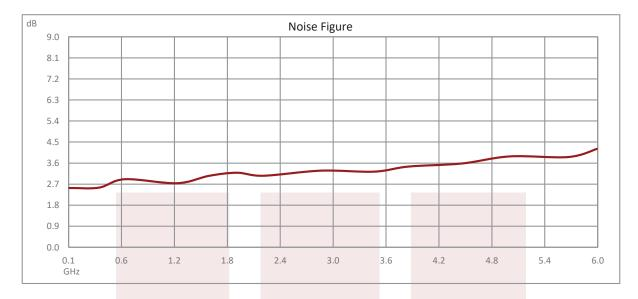
3.5 dB NF Input Protected Low Noise Amplifier, Operating from 10 MHz to 6 GHz with 30 dB Gain, 16.5 dBm Psat and SMA from Fairview Microwave is in-stock and available to ship same-day. All of our RF/microwave products are available off-the-shelf from our ISO 9001:2008 certified facilities in Lewisville, Texas. Fairview Microwave is RF on-demand.
