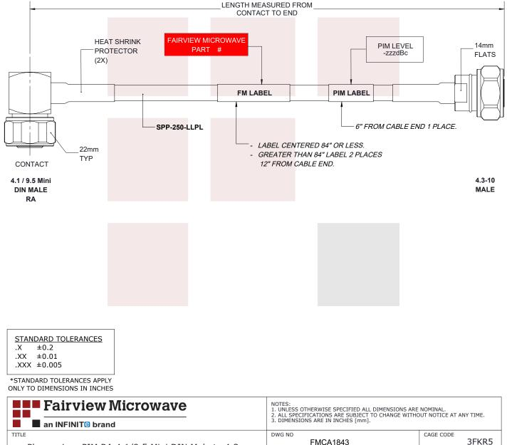
Plenum Low PIM RA 4.1/9.5 Mini DIN Male to 4.3-10 Male Cable SPP-250-LLPL Coax Using Times Microwave Parts
