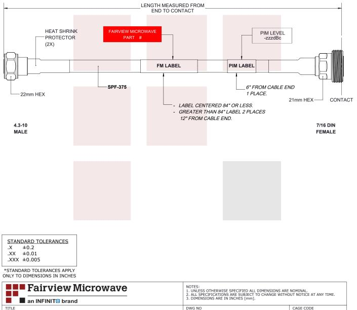
Fire Rated Low PIM 4.3-10 Male to 7/16 DIN Female Cable SPF-375 Coax Using Times Microwave Parts
