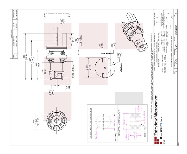
75 Ohm 12G SDI HD-BNC Female Bulkhead PCB Connector 0.062" Board Thickness Solder Attachment
