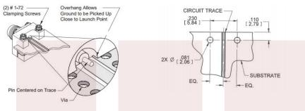
Step 3: Verify that the transition block is secured on the board.
