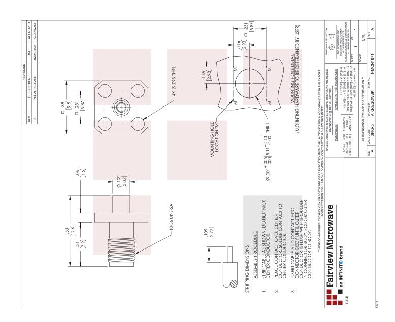
SSMA Female Connector Solder Attachment 4 Hole Flange for FM-SR086ALTN, FM-SR086TB, RG405, .232 inch Hole Spacing
