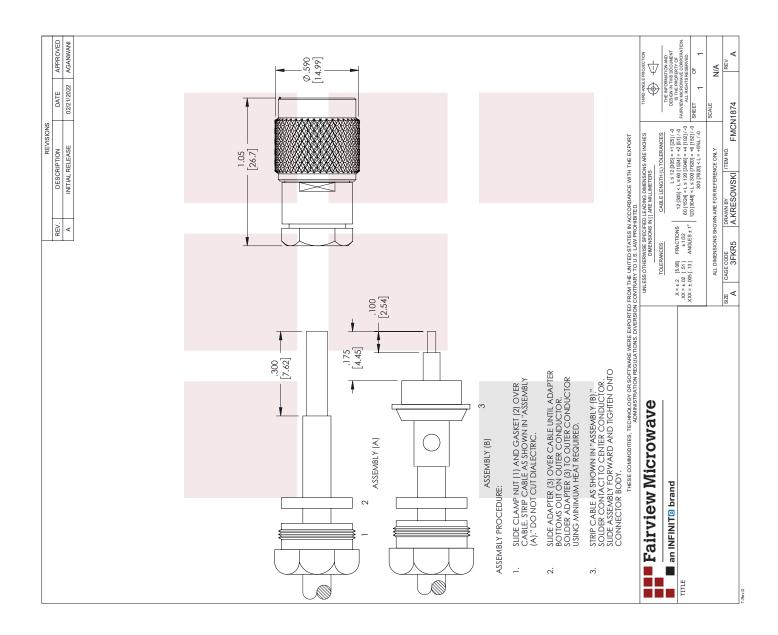
TNC Male Connector Clamp/Solder Attachment for FM-SR086ALTN, FM-SR086TB, RG405
