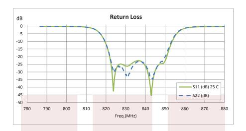
Bandpass Cavity Filter Operating From 824 MHz to 849 MHz With SMA Female Connectors from Fairview Microwave is instock and available to ship same-day. All of our RF/microwave products are available off-the-shelf from our ISO 9001:2008 certified facilities in Allen, Texas. Fairview Microwave is RF on-demand.
