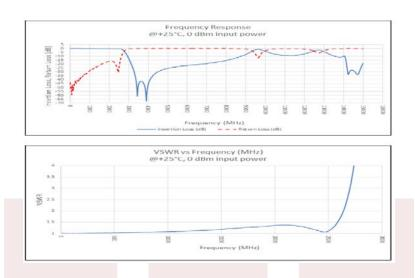
DC to 2500 MHz SMA Low Pass Harmonic Filter, 50W Pin, L & S Bands, 0.3 dB Loss and > 25 dB Rejection from Fairview Microwave is in-stock and available to ship same-day. All of our RF/microwave products are available off-the-shelf from our ISO 9001:2008 certified facilities in Lewisville, Texas. Fairview Microwave is RF on-demand.
