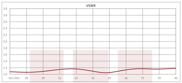
WR-28 to 2.92mm Female Waveguide to Coax Adapter UG-599/U Square Cover Flange With 26.5 GHz to 40 GHz Frequency Range For Ka Band from Fairview Microwave is in-stock and available to ship same-day. All of our RF/microwave products are available off-the-shelf from our ISO 9001:2008 certified facilities in Allen, Texas. Fairview Microwave is RF on-demand.
