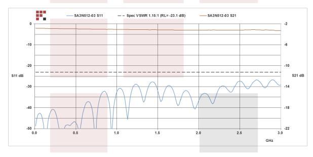
3 dB Fixed Attenuator N Male To N Female Up To 3 GHz Rated To 50 Watts With Black Aluminum Heatsink Body from Fairview Microwave is in-stock and available to ship same-day. All of our RF/microwave products are available off-the-shelf from our ISO 9001:2008 certified facilities in Lewisville, Texas. Fairview Microwave is RF on-demand.
