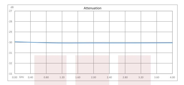
30 dB Fixed Attenuator SMA Male To SMA Female Up To 4 GHz Rated To 25 Watts With Black Aluminum Heatsink Body from Fairview Microwave is in-stock and available to ship same-day. All of our RF/microwave products are available off-the-shelf from our ISO 9001:2008 certified facilities in Allen, Texas. Fairview Microwave is RF on-demand.
