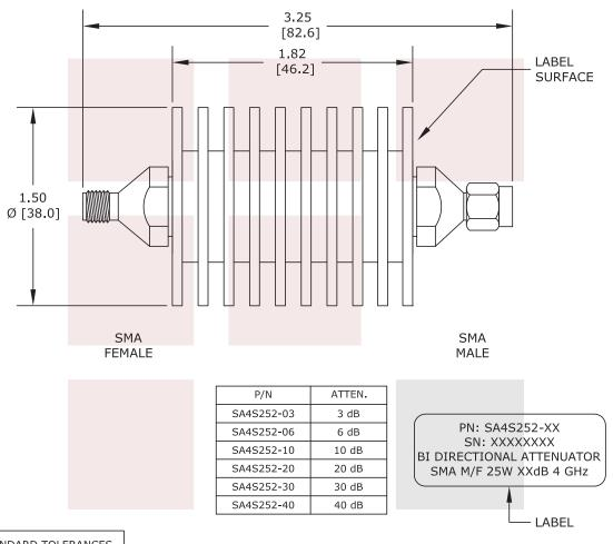
STANDARD TOLERANCES DIMENSIONS IN INCHES AND TOLERANCE ±0.08%
