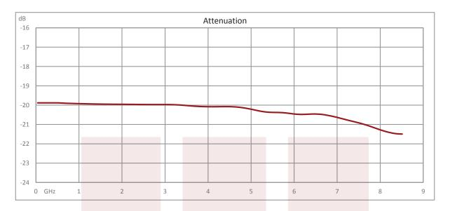
20 dB Fixed Attenuator N Male to N Female Directional Up to 8.5 GHz Rated to 250 Watts with Black Aluminum Heatsink Body from Fairview Microwave is in-stock and available to ship same-day. All of our RF/microwave products are available off-the-shelf from our ISO 9001:2008 certified facilities in Lewisville, Texas. Fairview Microwave is RF on-demand.
