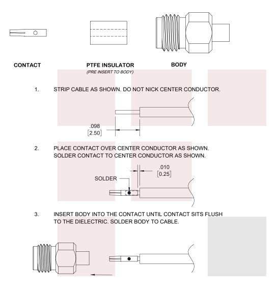
SMA Female Connector Solder/Non-Solder Contact Attachment For RG405, RG405 Tinned, .086 SR Cable from Fairview Microwave is in-stock and available to ship same-day. All of our RF/microwave products are available off-the-shelf from our ISO 9001:2008 certified facilities in Allen, Texas. Fairview Microwave is RF on-demand.
