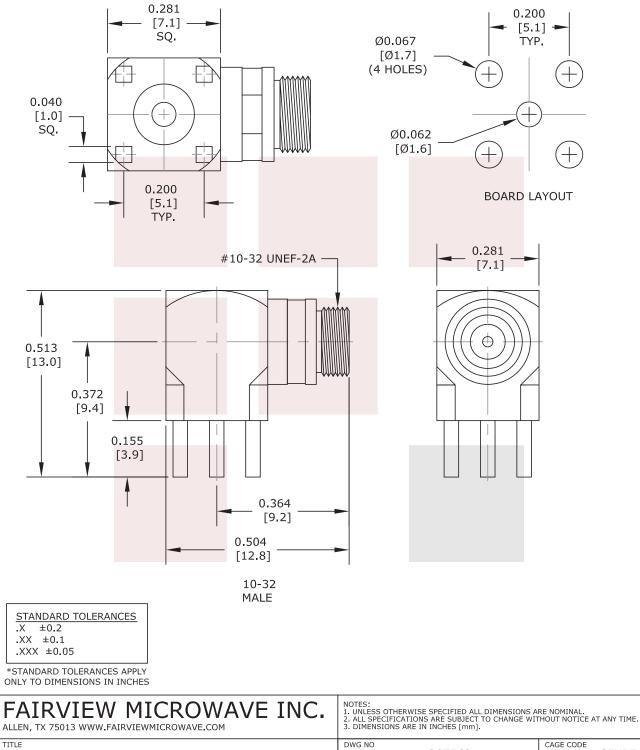
RA 10-32 Female PCB Connector Thru Hole Solder Attachment
