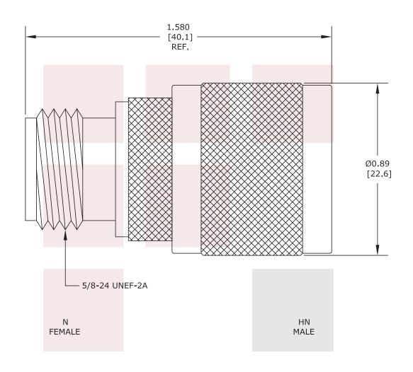
$\begin{array}{cc} \underline{\text{STANDARD TOLERANCES}} \\ .X & \pm 0.2 \\ .XX & \pm 0.1 \end{array}$
